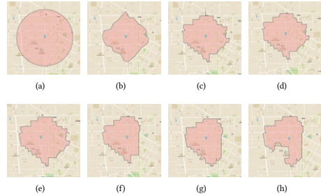
Figure 12: Results of Single Delivery Scope Drawing Algorithm: (a) Initialization with Shifted Center Point (b) Navigation Distance Modification (c) Navigation Route Process (d) Remove Stub (e) Scope Compression Process (f) Shipping Scope Intersection (g) Merge High-Demand Areas (h) Remove Improper Location 2
