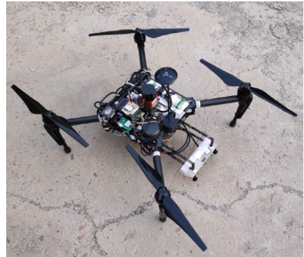
Figure 2. The device we used for our dataset. It contains oblique top-down global shutter stereo camera( AR0135, 30Hz) with 752×480 resolution and it contains a build-in IMU ( ICM20602, 500Hz ).
