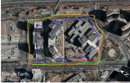
Figure 4. The estimated trajectories with good initial stereo extrinsic in hand held outdoor environment aligned to Google Map. VINS-Fusion (red), S-MSCKF (blue), our method (yellow) and GPS (green).
